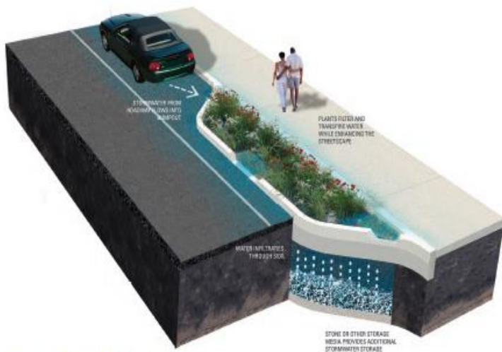
Midblock Stormwater Curb Extension
