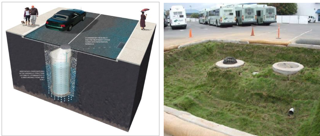
Figure 2-39. Conceptual example of a dry well located in a street and a dry well located in a bioretention area in a corporation yard in Elk Grove, CA. (Courtesy of PWD and the City of Elk Grove)
