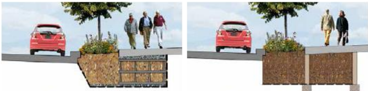
Figure 2-31. Stormwater tree well filter conceptual examples: modular suspended pavement system (left), column suspended pavement system (right). (Courtesy of PWD)
