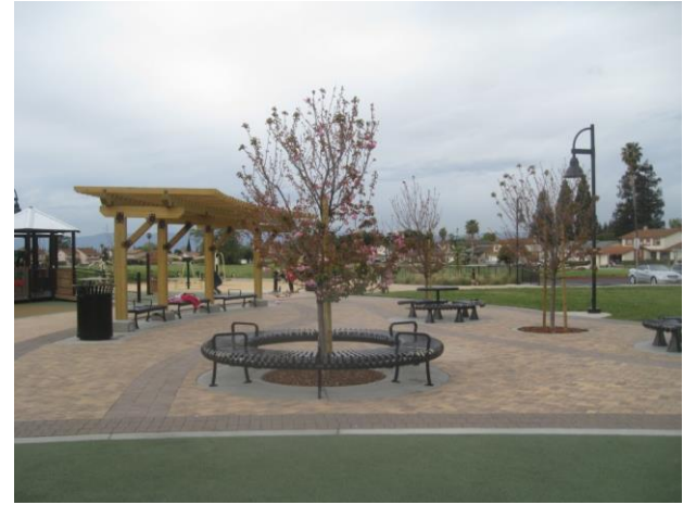
Figure 6-21. Commodore Park integrates various types of pervious pavement and vegetated areas into a beautiful and functional park. (Credit: San Jose)
