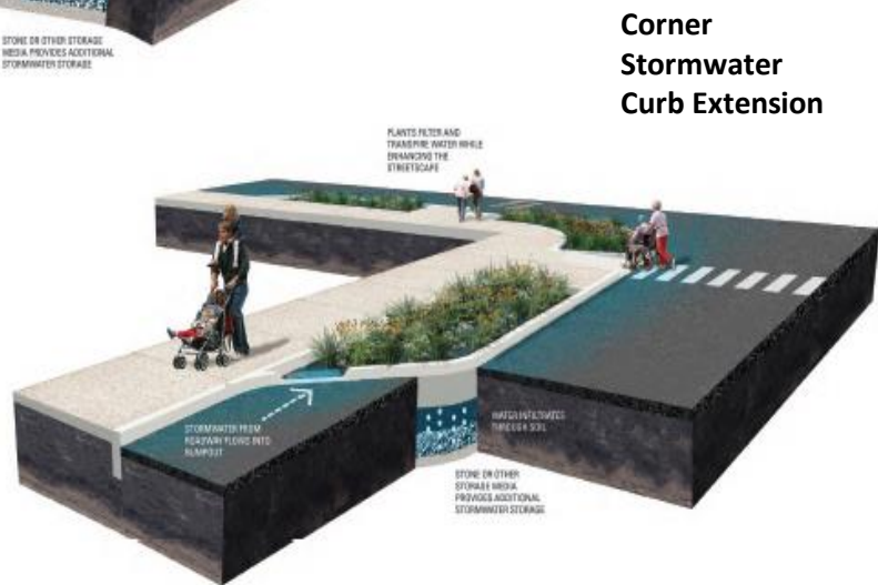
Figure 2-24. Conceptual examples of midblock (top left) and corner (bottom right) stormwater curb extensions. (Courtesy of PWD)
