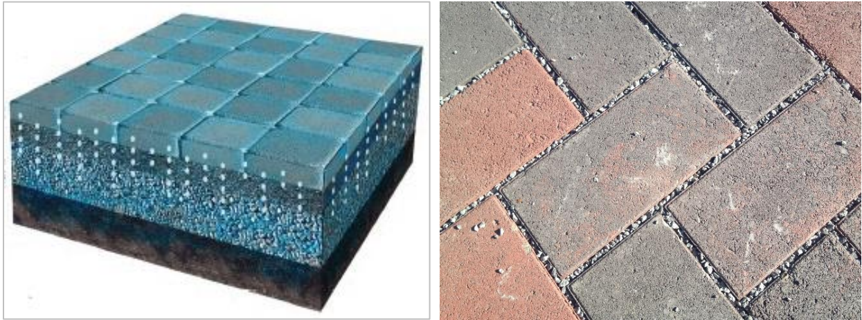
Figure 2-35. Permeable interlocking concrete pavers conceptual example (left) and Allston Way in Berkeley (right). (Courtesy of PWD (left) and EOA (right))
