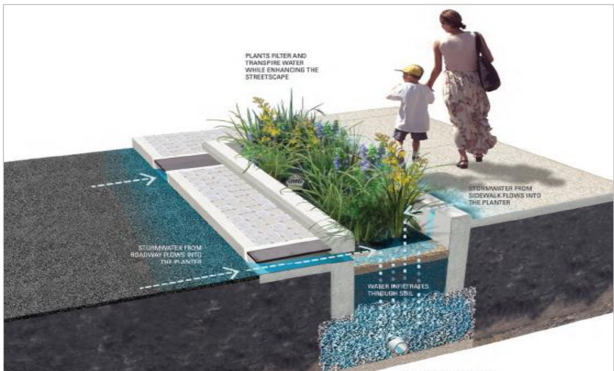
Figure 2-21. Conceptual stormwater planter with vertical sides. (Courtesy of PWD)
