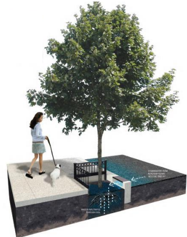
Figure 2-29. Stormwater tree well filter, conceptual example. (Courtesy of PWD)
