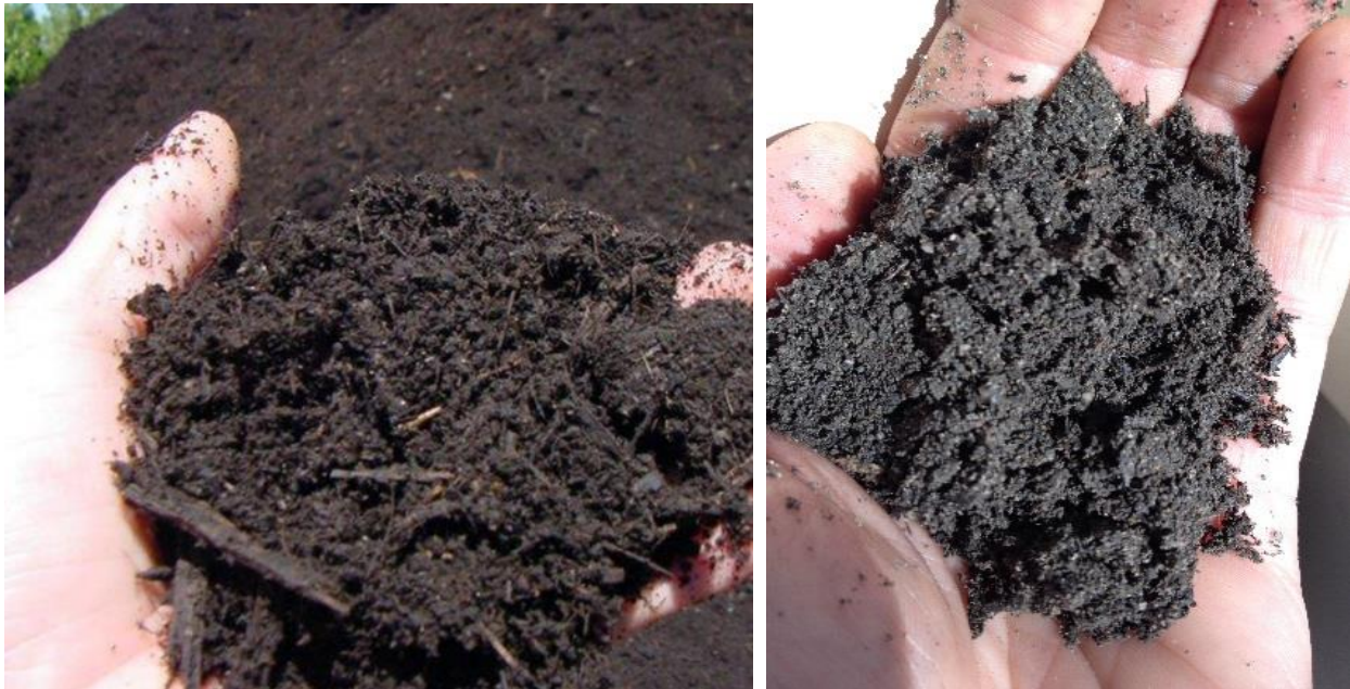
Figure 3-49. Compost (left) mixed with sand produces the mix (right) in the Biotreatment Soil Media. (Credit: EOA)
