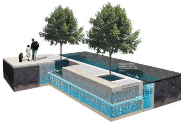
Figure 2-29. Stormwater tree well filter, conceptual example. (Courtesy of PWD)
