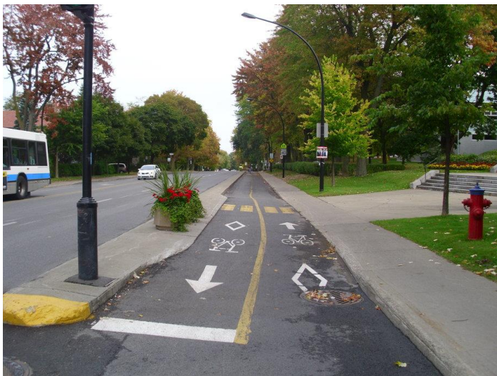
Figure 3-14. Cycletrack in Montreal on Chemin de la Côte Sainte Catherine with landscaping behind the adjacent sidewalk that could have been used for GSI measures. (Credit: dandyhorsemagazine.com)
