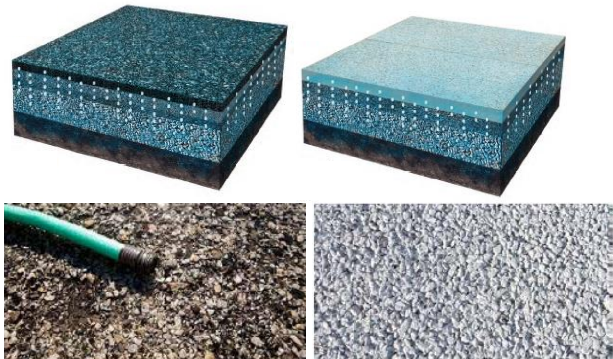
Figure 2-33. Conceptual examples of porous asphalt (top left) and pervious concrete (top right), and photographs of porous asphalt (bottom left) and pervious concrete (bottom right). (Courtesy of PWD (top) and DDOT (bottom))
