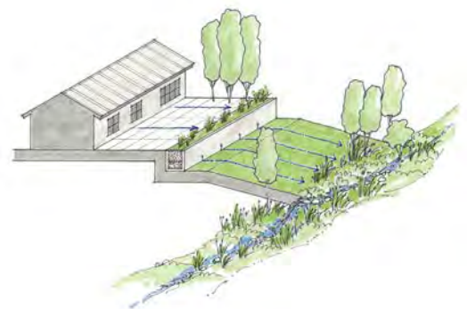
Flow-through planter built into a hillside. Flows from the underdrain and overflow must be directed in accordance with local requirements.
